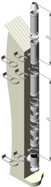
**CONFIGURACION 5: ANCLAJE RECORTABLE LARGO 845 / ANCLAJE RECORTABLE LARGO PLANO 846**
