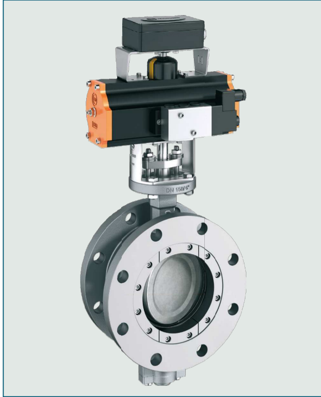
Double-Zanged butterfly valve in double-eccentric construction. Reliable sealing even with extreme temperature and pressure conditions.
