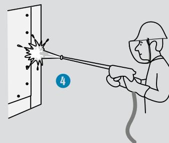
4. Remove pickling residues by using a high-pressure water jet, or with a stain-less steel brush and then rinse with water. The waste water should be treated before discharge.
